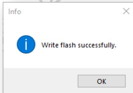
10. Confirm by clicking on the OK button before you remove the micro-USB cable from the GD-73, and power cycle the radio by pressing the on / off button to return to normal. The update process is now complete.
